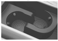
Push the button. The cup supporter protrudes from the front console. Push in the cup supporter after use.
