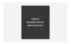
When the outside rearview mirror warning light is not working properly, the "Check side view mirror warning light" (or "Check outside mirror warning icon") warning message will appear on the instrument cluster for several seconds, and the master (△) warning light will appear on the instrument cluster. If this occurs, we recommend that your vehicle be inspected by an authorized HYUNDAI dealer.
