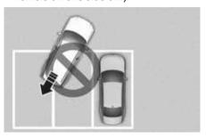
If Remote Smart Parking Assist is used, when parking in a parking space with a vehicle only on one side, your vehicle may cross the parking line to avoid the parked vehicle.
