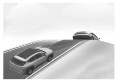
During uphill or downhill coasting, the smart recuperation system may not detect a moving vehicle in your lane, and cause your vehicle to accelerate. Also, your vehicle speed decelerates when a vehicle ahead is detected suddenly. Apply the brake pedal or accelerator pedal depending on the road and driving conditions.
