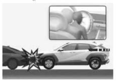
Front airbags are designed to inflate in a frontal collision depending on the severity of impact.
