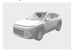
[A] Front view camera See the illustration above for the detailed location of the detecting sensors.
