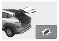
The cargo area lamp turns on when the tailgate is opened and off when the tailgate is closed.
