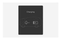
The high voltage battery is charged up by the regenerative brake system. (Wheel  $\rightarrow$  Battery)
