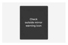
When the outside rearview mirror warning light is not working properly, the "Check side view mirror warning light" (or "Check outside mirror warning icon") warning message will appear on the instrument cluster for several seconds, and the master (△) warning light will illuminate on the cluster. If this occur, we recommend that your vehicle be inspected by an authorized HYUNDAI dealer.
