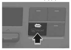
Press the A/C button to manually turn on the system on (indicator light ON) and off.
