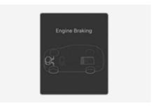
The engine braking is used to decelerate the vehicle. (Wheel → Engine)
