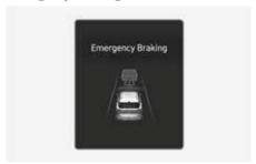
To warn the driver that emergency braking will be assisted, the "Emergency Braking" warning message appears and the ( ) warning light blinks on the cluster with warning sound and haptic feedback of the steering wheel (if equipped).
