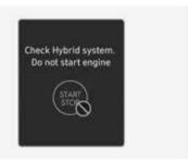
This message appears when the hybrid battery power (SOC) level is low. A warning chime will sound until the problem is solved. Refrain from driving when the warning message appears.
