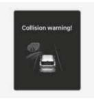
To warn the driver of a collision, the "Collision warning!" warning message appears and the ( ) warning light blinks on the cluster with warning sound and haptic feedback of the steering wheel (if equipped).
