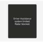
When the front windshield where the front view camera is located, front radar cover, or sensor is covered with foreign material, such as snow or rain, it can reduce the detecting performance and temporarily limit or disable Forward Collision-Avoidance Assist.
