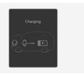
The engine charges the high voltage battery according to the vehicle and surrounding conditions.
