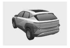
[A] Rear corner radar Refer to the illustration above for the detailed location of the detecting sensors.
