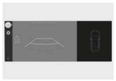
To warn the driver of an approaching vehicle from the rear left/right side of your vehicle, the warning light on the outside rearview mirror will blink and a warning will appear on the cluster. At the same time, an audible warning will sound. If Rear View Monitor is operating, a warning will also appear on the infotainment system.
