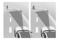
Forward Collision-Avoidance Assist may not detect a vehicle, a powered two wheeler, a pedestrian or a cyclists in front of you when driving on curved roads adversely affecting the performance of the sensors. This may result in no warning, braking assist when necessary.
