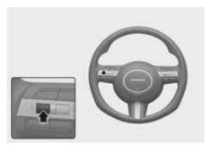
Press the IIO switch to temporarily pause the set speed limit. The set speed limit will turn off but the Speed Limit (Start) indicator will stay on.
