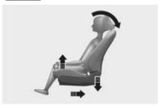
Relaxation comfort seats distribute body pressure and concentrated weight on specific body parts that occur while sitting in the same position for a long period of time. The seat relieves fatigue and discomfort by providing the optimal sit position.
