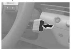
To shift the gear to P (Park), press the P button while depressing the brake pedal. If you turn the engine off in R (Reverse), N (Neutral) or D (Drive), the gear will automatically shift to P (Park).
