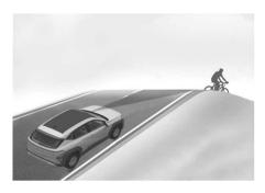
Forward Collision-Avoidance Assist may not detect a vehicle, a powered two wheeler, a pedestrian or a cyclists in front of you while driving uphill or downhill, adversely affecting the performance of the sensors.
