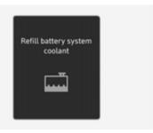
This message appears when the battery system coolant is nearly empty. You should refill the battery system coolant.
