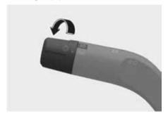
The headlight, position light, license plate light and instrument panel lamp are turned ON.
