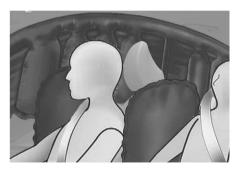
Side and curtain airbags are designed to inflate when an impact is detected by side collision sensors depending on the severity of impact resulting from a side impact collision.
