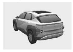
[A] Rear corner radar See the illustration above for the detailed location of the detecting sensors.
