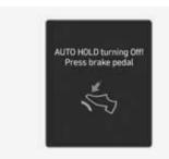
When the conversion from Auto Hold to EPB is not working properly, a warning sounds and a message appears.
