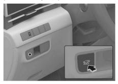
When the tailgate is closed, press the power tailgate open/close button. The power tailgate opens with a warning sound.
