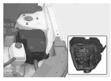
Inside the fuse panel cover, you can find the label describing fuse names and ratings.
