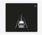
If the vehicle ahead and/or both lane markings are detected and your vehicle speed is below 200 km/h (120 mph), the green (a) indicator light appears on the cluster, and Lane Following Assist helps center the vehicle in the lane by assisting the steering wheel.
