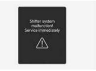
This message appears when the transmission or the shift dial does not properly operate in the P (Park) position.
