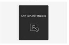
This message appears when the gear is shifted to P (Park) while the vehicle is moving.
