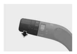
To flash the high beam headlight, pull the lever towards you, then release the lever. The high beams remains ON as long as you hold the lever towards you.
