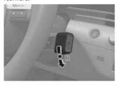
To shift the gear to R (Reverse), rotate the rotary gear shift dial to R (Reverse) while depressing the brake pedal.
