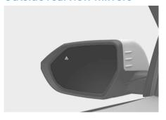
Your vehicle is equipped with both left-hand and right-hand outside rearview mirrors. The mirrors can be adjusted with the mirror adjustment control switch. Adjust the side view mirrors to your desired position before driving. The outside rearview mirrors can be folded to help prevent damage when going through an automatic car wash or when passing through a narrow street.
