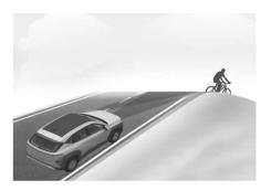
Forward Collision-Avoidance Assist may not detect a vehicle, a powered two wheeler, and a pedestrian or a cyclist in front of you while driving uphill or downhill, adversely affecting the performance of the sensors.
