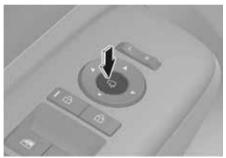
The outside rearview mirrors can be folded or unfolded by pressing the button.
