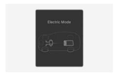
Only the motor power is used to drive the vehicle. (Battery  $\rightarrow$  Wheel)
