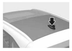
The shark fin antenna receives transmitted data (for example, AM/FM, SXM).
