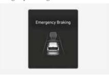
To warn the driver that emergency braking will be assisted, the "Emergency Braking" warning message appears and the ( ) warning light blinks on the cluster with warning sound and haptic feedback of the steering wheel (if equipped).
