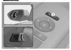
When the gear is shifted to the R (Reverse) position, the outside rearview mirrors rotate downwards to aid with driving in reverse.
