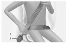
Pull the belt out of the retractor and insert the metal tab (1) into the buckle (2). There An audible "click" sounds when the tab locks into the buckle. Make sure the seat belt is not twisted.
