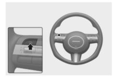
Press the Driving Assist button to turn Cruise Control off. The Cruise (Notes) indicator will go off.
