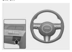
With the vehicle on, shortly press the Lane Driving Assist button located on the steering wheel to turn on Lane Following Assist. The grey or green (a) indicator light will appear on the cluster.
