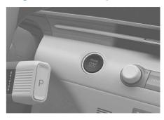
Whenever the front door is opened, the Start Engine Start/Stop button illuminates and goes off for a few seconds after the door is closed.
