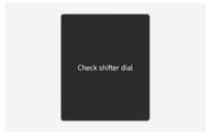
This message appears when there is a malfunction with the rotary gear shift dial.
