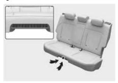
The hybrid battery cooling duct is located below the center of the rear seat. The cooling duct cools down the hybrid battery. When the hybrid battery cooling duct is blocked, the hybrid battery may be overheated.
