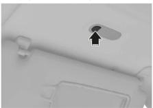
Push the switch to turn the lamp on or off.
