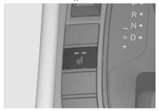
When the Engine Start/Stop button is in the ON position or when the engine is running, press the steering wheel heater button to warm the steering wheel.
