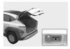
When the tailgate is closed, press the power tailgate open/close button to open the tailgate.
