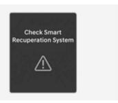
If the rear radar is covered by any foreign material, such as snow, rain, or dirt, the detecting performance may decrease and disable the smart recuperation system.
