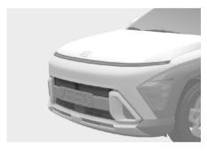
Active air flap system controls the air flap below the front bumper to cool the vehicle parts and improve energy efficiency.
