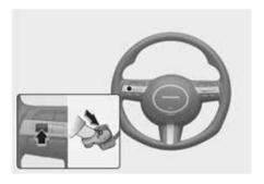
Press the IDswitch or depress the brake pedal to temporarily cancel Smart Cruise Control.
