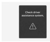
When Lane Following Assist is not working properly, the "Check Driver Assistance system" warning message will appear on the instrument cluster for several seconds, and the master (4) warning light appears on the instrument cluster. If this occur, we recommend that your vehicle be inspected by an authorized HYUNDAI dealer.
