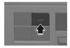
Press the OFF button to turn the climate control system off. You can still operate the mode and air intake buttons as long as the Engine Start/Stop button is in the ON position.
