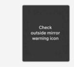
When the outside rearview mirror warning light is not working properly, the "Check outside mirror warning icon" warning message will appear on the cluster for several seconds, and the master warning light (△) will appear on the cluster. If this occurs, we recommend that your vehicle be inspected by an authorized HYUNDAI dealer.
