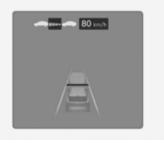
If you want to speed up temporarily without altering the set speed while Smart Cruise Control is operating, depress the accelerator pedal. While the accelerator pedal is depressed, the set speed, distance level and target distance will blink on the cluster.
