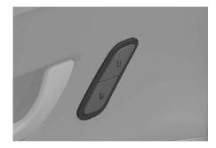
The Integrated Memory System for the driver's seat is equipped on some models and allows the driver to store and recall the following memory settings with a simple button operation.
