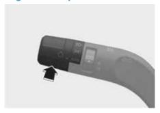
To turn on the high beam headlight, push the lever away from you. The lever returns to its original position.
