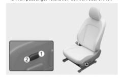
To activate relaxation comfort seat Press the switch (1), an alarm appears on the infotainment system. Then, press the switch (1) again.
