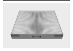
Install a new cabin air filter in the correct direction with the arrow symbol ( $\downarrow$ ) facing downwards, to prevent noise and reduce effectiveness
