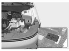
High voltage cut-off switch is a device located inside the engine compartment to block the battery's high voltage when your vehicle is inspected at an authorized HYUNDAI dealer.
