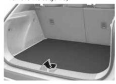
Remove the top board and insert the top board all the way in along the lower groove on both sides.
