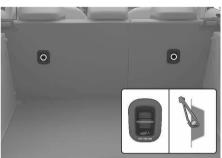
First secure the child restraint with the ISOFIX anchorages or the seat belt. If the child restraint manufacturer recommends that the top tether strap be attached, attach and tighten the top tether strap to the top tether strap anchorage.
