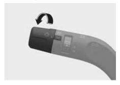
The position light, license plate light and instrument panel lamp are turned ON.
