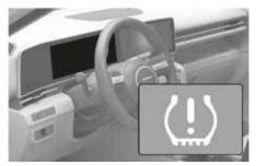
The TPMS Malfunction Indicator (Ш) illuminates after it blinks for approximately one minute when there is a problem with the Tire Pressure Monitoring System.
