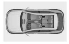
The driver's and front passenger's seats are equipped with adjustable headrests for the passengers safety and comfort.
