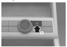
Press the Parking/View button (1) while the gear is in P (Park), D (Drive) or N (Neutral) to turn on the Rear View Monitor.
