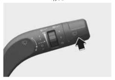
The rear window washer switch is located at the end of the washer switch lever.
