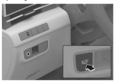
When the tailgate is closed, press the tailgate open button. The tailgate opens.
