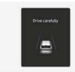
When the vehicle is stopped due to emergency braking, the "**Drive carefully**" warning message will appear on the cluster.
