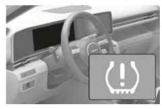
The TPMS malfunction indicator ((!)) illuminates after blinking for about 70 seconds when there is a problem with the Tire Pressure Monitoring System.
