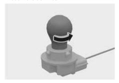
6. Install a new bulb and reinstall in the reverse order.
