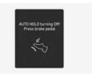
When the conversion from Auto Hold to EPB is not working properly, a warning sounds and a message appears.
