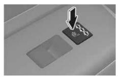
While the engine is running, press the seat warmer switch to warm the rear seat.
