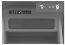
Insert the key or a similar rigid device into the passenger's front airbag ON/OFF switch and turn it to the ON position [A]. The passenger airbag ON indicator (S) illuminates.
