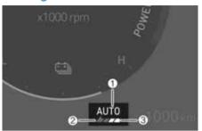
When the smart recuperation system is ON, the regenerative braking level appears as "AUTO" on the instrument cluster. The "AUTO" appears in grey in the ready state. The system automatically controls the regenerative braking level (2) according to the smart recuperation system operating conditions. If the front radar detects a vehicle in front, the indicator light (3) appears in green.
