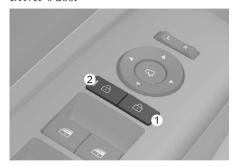
When pressing the figure portion (1) on the switch, all vehicle doors are locked.
