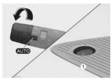
The position light and headlight may be turned ON or OFF automatically depending on the amount of daylight as measured by the ambient light sensor (1) at the upper end of the windshield glass.
