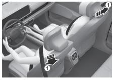
Retractor pre-tensioner seat belt / Front seat and rear outboard seat
