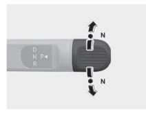
To shift the gear to N (Neutral), rotate the rotary gear shift dial to N (Neutral) while depressing the brake pedal.
