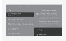
With the vehicle on, select "**Setup** (Settings) > Vehicle > Driver assistance > Warning volume" from the Settings menu to change the Warning Volume.
