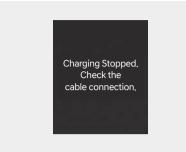
This warning message is displayed when charging is stopped because the charging connector is not correctly connected to the charging inlet
