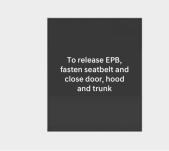
To release EPB, fasten seatbelt and close door, hood and trunk
