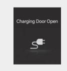
This message is displayed when the vehicle is driven with the charging door opened. Close the charging door and then start driving.
