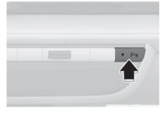
Press the Parking Safety (P<sub>w</sub>) button to turn on Forward/Reverse Parking Distance Warning. Press the button again to turn off the function.
