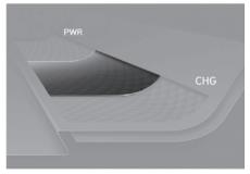
The Power/Charge Gauge shows the energy consumption rate of the vehicle and the
