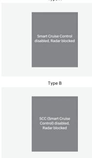
When the front radar cover or sensor is covered with snow, rain, or foreign material, it can reduce the detecting performance and temporarily limit or disable Smart Cruise Control.
