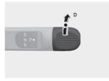
To shift the gear to D (Drive), rotate the rotary gear shift dial to D (Drive) while depressing the brake pedal.
