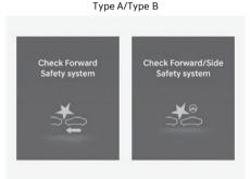
When Forward Collision-Avoidance Assist is not working properly, the 'Check Forward Safety system(s)' and 'Check Forward/Side Safety system(s)' warning message will appear, and the A, and warning lights will illuminate on the instrument cluster. We recommend that you have the vehicle inspected by an authorized HYUNDAI dealer.
