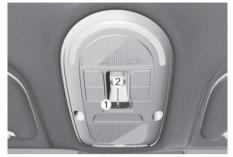
Elements of the UAE eCall System, installed in passenger compartment: (1) SOS button (2) LED
