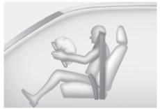
When the SRSCM detects a sufficiently severe impact to the front of the vehicle, it will automatically deploy the front airbags.
