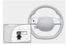
Press the IIO switch to temporarily pause the set speed limit. The set speed limit will turn off but the Speed Limit (RILMIT) indicator will stay on.
