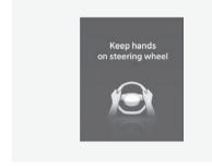
If the driver takes their hands off the steering wheel for several seconds, the "Keep hands on steering wheel" warning message will appear on the cluster, and an audible warning will sound in stages.
