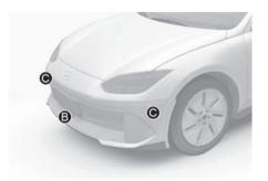
The front view camera and front radar are used as a detecting sensor to detect front vehicles.
