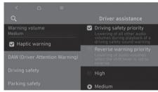
With the vehicle on, select 'Setup (Settings) > Vehicle > Driver assistance > Warning volume' from the Settings menu to change the Warning volume for Forward Collision-Avoidance Assist. Even though 'Off' is selected for Warning volume, Warning volume will not turn off but sound as 'Low' is selected.
