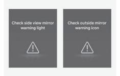
When the outside rearview warning light is not working properly, the "Check side view mirror warning light" (or "Check outside mirror warning icon") warning message will appear on the instrument cluster for several seconds, and the master ( $\triangle$ ) warning light will illuminate on the instrument cluster. If this occurs, we recommend that you have the vehicle inspected by an authorized HYUNDAI dealer.
