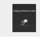
This message is displayed when you start the vehicle without unplugging the charging cable. Unplug the charging cable, and then turn on the vehicle.
