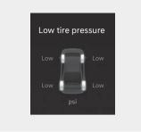
This warning message is displayed if the tire pressure is low. The corresponding tire on the vehicle will be illuminated.
