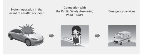
The Pan-European eCall device automatically makes an emergency call to the Public Safety Answering Point (PSAP) for proper rescuing operations in event of vehicle accident.
