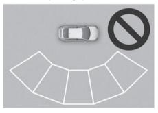
Remote Smart Parking Assist does not work properly when the parking lines are not parallel. Do not park although the parking space is recognized by the sensor. Inclined parking space
