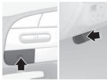
Press the IIO switch or depress the brake pedal to temporarily cancel Smart Cruise Control.
