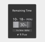
This message is displayed to notify the remaining time to charge the battery to the selected target battery charge level.
