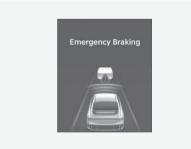
To warn the driver that emergency braking will be assisted, Forward Safety waring light ((1) blinking, the 'Emergency Braking' warning message will appear on the cluster, an audible warning will sound and the steering wheel will vibrate. Emergency braking will operate under the following conditions.
