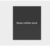
This message is displayed when the rotary gear shift dial does not return back to it's normal position after rotating it.
