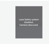
When the front windshield where the front view camera is located, or sensor is covered with foreign material, such as snow or rain, it can reduce the detecting performance and temporarily limit or disable Lane Keeping Assist.
