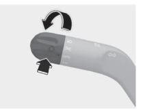
High Beam Assist will automatically adjust the headlamp range (switches between high beam and low beam) depending on the brightness of detected vehicles and certain road conditions.
