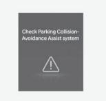
When Parking Collision-Avoidance Assist or other related functions are not working properly, the 'Check Parking Collision-Avoidance Assist system' warning message will appear on the instrument cluster, and Parking Collision-Avoidance Assist will turn off automatically. We recommend that you have the vehicle inspected by an authorized HYUNDAI dealer.
