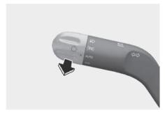
To flash the high beam headlamp, pull the lever towards you, then release the lever. The high beams will remain ON as long as you hold the lever towards you.
