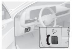
Manual type (if equipped) To adjust the headlamp beam level according to the number of the passengers and loading weight in the luggage area, turn the beam leveling switch.
