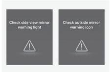
When the outside rearview mirror warning light is not working properly, the 'Check side view mirror warning light' (or 'Check outside mirror warning icon') warning message will appear on the instrument cluster for several seconds, and the master ( $\triangle$ ) warning light will illuminate on the cluster. If this occur,
