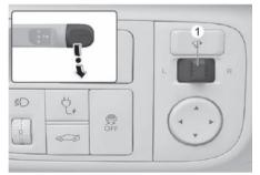
Use the DSM camera selection lever (1) to select L (Left) or R (Right).
