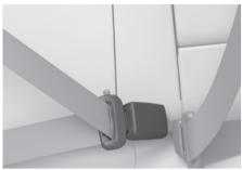
When using the rear center seat belt, the buckle with the "CENTER" mark must be used.
