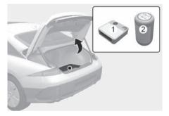
For safe operation, carefully read and follow the instructions in this manual before use. (1) Compressor (2) Sealant bottle
