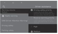
With the vehicle on, select "Setup (Settings) > Vehicle > Driver assistance > Warning volume" from the Settings menu to change the Warning volume for Safe Exit Warning.
