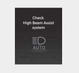
When High Beam Assist is not working properly, the 'Check High Beam Assist system' warning message will appear and warning light will illuminate on the cluster. We recommend that the function be inspected by an authorized HYUNDAI dealer.
