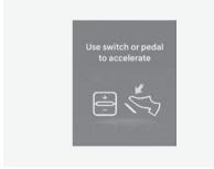
In traffic, your vehicle will stop if the vehicle ahead of you stops. Also, if the vehicle ahead of you starts moving, your vehicle will start as well. In addition, after the vehicle has stopped and a certain time have passed, the "Use switch or pedal to accelerate" message will appear on the instrument cluster. Depress the accelerator pedal or operate the + switch, - switch or IID switch to start driving.
