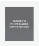
When the front windshield where the front view camera is located is covered with foreign material, such as snow or rain, it can reduce the detecting performance and temporarily limit or disable Intelligent Speed Limit Assist. If this occurs, the "Speed Limit system disabled. Camera obscured" warning message and (⊖) warning light will appear on the instrument cluster.
