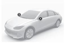
[A] Wide-side view camera (camera located at bottom of the mirror)
