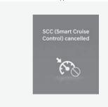
• The vehicle speed is above 210 km/h (130 mph)
