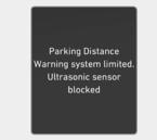
If this occurs the "Parking Distance Warning system limited. Ultrasonic sensor blocked" warning message appears on the instrument cluster. Parking Distance Warning will operate properly when snow, rain or foreign material is removed. If Parking Distance Warning does not operate properly after obstruction (snow, rain, or foreign material) is removed (including trailer, carrier, etc., from the rear bumper), have the vehicle inspected by an authorized HYUNDAI dealer.
