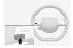
With the vehicle on, shortly press the Lane Driving Assist button located on the steering wheel to turn on Lane Following Assist. The grey or green  $(\bigcirc)$  indicator light will illuminate on the cluster.
