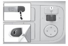
When the gear is shifted to the R (Reverse) position, the outside rearview lever(s) will rotate downwards to aid with driving in reverse.
