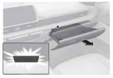
Opening the glove box comes on the lamp. When the glove box is not closed completely, the lamp may keep coming on.
