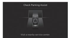
When Remote Smart Parking Assist is not working properly, the 'Check Parking Assist' warning message will appear on the infotainment system screen. If the message appears, stop using Remote Smart Parking Assist, and we recommend that you have the vehicle inspected by an authorized HYUNDAI dealer.
