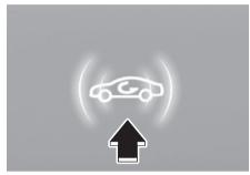
Air intake control is used to select either Fresh mode (outside air) or Recirculation mode (cabin air).
