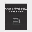
When the high voltage battery level reaches below about 5 %, this warning message is displayed.
