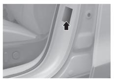
The vehicle certification label attached on the driver's (or front passenger's) side center pillar gives the vehicle identification number (VIN).
