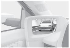
The digital side mirrors are a replacement for the outside rearview mirrors and help with changing lanes by displaying the rear view image on the monitors inside the vehicle.
