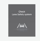
When Lane Keeping Assist is not working properly, the "Check Lane Safety system" warning message will appear and the yellow (AN) indicator light will illuminate on the cluster. If this occurs, we recommend that you have the vehicle inspected by an authorized HYUNDAI dealer.
