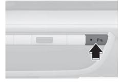
Press the Parking Safety (P<sub>4</sub>) button to turn on Forward/Reverse Parking Distance Warning. Press the button again to turn off the function.
