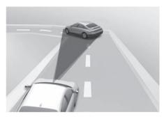
Your vehicle speed can be reduced due to a vehicle in the adjacent lane.
