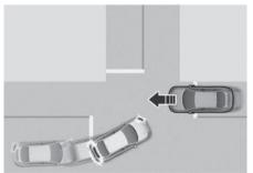
Junction Turning function can help avoid a collision with an oncoming vehicle in an adjacent lane when turning left (left-hand drive) or right (right-hand drive) at a crossroad with the turn signal on by applying emergency braking.
