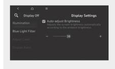
The brightness of the instrument panel can also be adjusted from the infotainment system screen. When Start/Stop button is in the ON position, select '**Settings** > **Display** > **Illumination**'.
