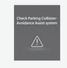
When Reverse Parking Collision-Avoidance Assist or other related functions are not working properly, the "Check Reverse Parking Collision-Avoidance Assist system" warning message will appear on the instrument cluster, and Reverse Parking Collision-Avoidance Assist will turn off automatically. We recommend that you have the vehicle inspected by an authorized HYUNDAI dealer.
