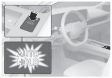
1 With the driver's door and hood closed, depress the brake pedal and then press the AUTO HOLD switch. The white AUTO HOLD indicator will come on and the system will be in the standby position.
