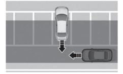
Rear Cross-Traffic Collision-Avoidance Assist may detect vehicles passing by behind you when parking in reverse into a parking space. If this occurs, the function may unnecessarily warn the driver and control the brake.
