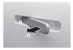
Push the button on the front outside door handle (the engraved part) while carrying the Smart Key with you, all doors will unlock.
