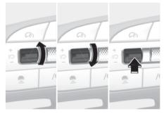
To resume Manual Speed Limit Assist after the function was paused, operate the +, -, IID switch.
