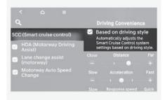
With the vehicle on, select "Setup (Settings) > Vehicle > Driver assistance > Driving Convenience > SCC (Smart Cruise Control) > Based on driving style" from the settings menu to check the driver's driving style, and to change each driving style manually.
