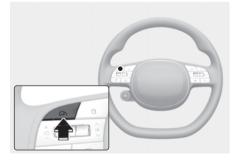
1 Press and hold Driving Assist (CR) button at the desired speed. The Speed Limit (SLIMT) indicator will illuminate on the cluster. 3. The set speed limit will be displayed on the cluster.
