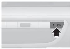
Turning Reverse Parking Collision Avoidance Assist On/Off
