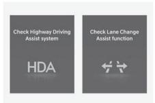
When Highway Driving Assist or Highway Lane Change function is not working properly, the "Check Highway Driving Assist (HDA) system" or "Check Lane Change Assist function" warning message will appear, and the ▲ warning light will illuminate on the cluster. We recommend that the vehicle be inspected by an authorized HYUNDAI dealer.
