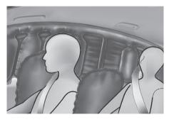
Side and curtain airbags and front center side airbag
