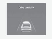
• When the vehicle is stopped due to emergency braking, the 'Drive carefully' warning message will appear on the cluster.
