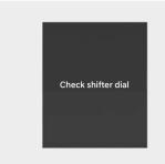
This message is displayed when there is a malfunction with the rotary gear shift dial.
