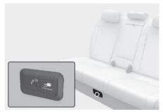
V2L(Vehicle to Load) is installed at the central rear seat. V2L is a convenient feature which provides enough electricity to use diverse household electrical appliances in the vehicle.
