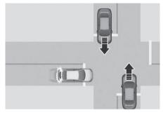
Junction Crossing function can help avoid a collision with oncoming vehicles on the left or right side when crossing an intersection by applying emergency braking.
