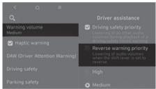
With the vehicle on, select "Setup (Settings) > Vehicle > Driver assistance > Warning volume > Reverse warning priority" from the Settings menu.
