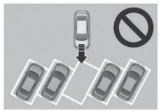
Remote forward function may not operate properly in a diagonal parking space.
