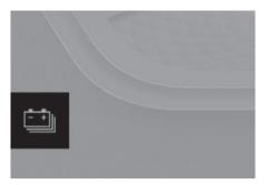
When the remaining battery is lower than 20 % on the SOC gauge, the warning light ( ) turns ON to alert you of the battery level.
