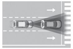
Forward Collision-Avoidance Assist is designed to help detect and monitor the vehicle ahead, powered two-wheeler, a pedestrian or cyclist in the roadway and warn the driver that a collision is imminent with a warning message and warning and application of emergency braking.
