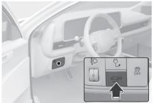
When the trunk is closed, press the power trunk open/close button. The power trunk will open with a warning sound.
