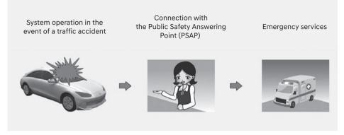
The UAE eCall device automatically makes an emergency call to the Public Safety Answering Point (PSAP) for proper rescuing operations in event of vehicle accident.
