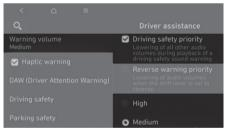
With the vehicle on, select "Setup (Settings) > Vehicle > Driver assistance > Warning volume" from the Settings menu to change the Warning volume.
