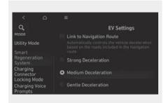
To adjust the regenerative braking level of the smart recuperation system, go to Settings (Setup) > EV > Smart recuperation (Smart regeneration system) from the infotainment system.
