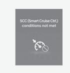
If the Driving Assist button, + switch, switch or **IIO** switch is operated when Smart Cruise Control operating conditions are nnot satisfied, the Smart Cruise Control conditions not met' (or'SCC'(Smart Cruise Ctrl.)) conditions not met' will appear on the cluster, and an audible warning will sound.
