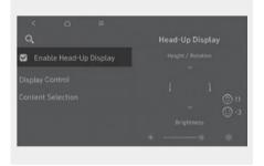
• Head-up display can be enabled from the Settings menu in the infotainment system screen.
