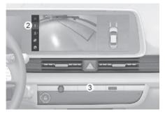
The front image is displayed on the screen when the gear is in N (Neutral) or D (Drive) to assist in parking. Using the view button (2) you may select top view, front view, side view.
