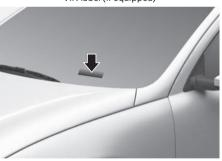
The VIN is also on a plate attached to the top of the left side dashboard. The number on the plate can easily be seen through the windshield from outside.
