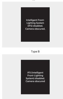
When Intelligent Front-Lighting System is not working properly, the 'Check Intelligent Front-Lighting System (IFS)' warning message will come on for a few second on the cluster. After the message disappears, the AFS and *(*) will illuminate on the cluster. We recommend that the system be inspected by an authorized HYUNDAI dealer.
