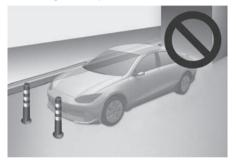
Remote Smart Parking Assist performance may reduce or collision with an obstacle may occur when there is a narrow object, circular pillar, square pillar, or a pillar surrounded by objects such as a fire extinguisher, etc., near the parking space. The driver should park the vehicle manually. · Paking next to a misaligned vehicle
