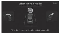
With the vehicle stopped by depressing the brake pedal, touch the infotainment system screen to select the desired exit direction.
