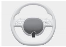
To sound the horn, press the area indicated by the horn symbol on your steering wheel
