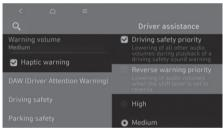
With the vehicle on, select "**Setup** (Settings) > Vehicle > Driver assistance > Warning volume" from the settings menu to change the Warning Volume for Blind-Spot Collision Avoidance Assist.
