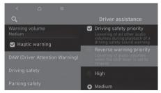
With the vehicle on, select "Setup (Settings) > Vehicle > Driver assistance > Warning volume" or "Setup (Settings) > Sound > Driver assistance" from the settings menu in the infotainment system to change the Warning Volume for Hands-off warning.
