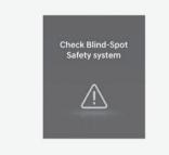
When Safe Exit Warning is not working properly, the "Check Blind-Spot Safety system(s)" warning message will appear on the instrument cluster for several seconds, and the master ((A)) warning light will illuminate on the instrument cluster. If this occurs, we recommend that you have the vehicle inspected by an authorized HYUNDAI dealer.
