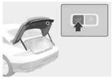
Press the power trunk close button. The trunk will close with a warning sound.
