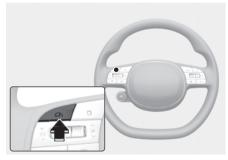
Press the Driving Assist ((C)) button to turn Cruise Control off. The Cruise ((C)CRUISE) indicator will go off.
