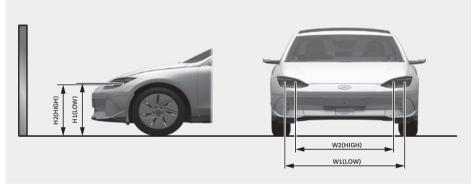
H1: Height between the head lamp bulb center and ground (Low beam)H2: Height between the head lamp bulb center and ground (High beam)W1: Distance between the two head lamp bulbs centers (Low beam)W2: Distance between the two head lamp bulbs centers (High beam)
