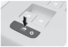
The driver can disable the power window switches on the rear passenger doors by pressing the power window lock button. When the power window lock button is pressed:
