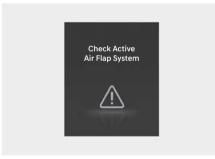
The active air flap system may not operate normally if the air flap is temporarily opened due to foreign factors or if the controller is contaminated by snow or rain, etc.
