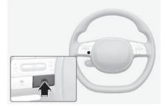
Whenever the engine is turned on,Lane Keeping Assist will always turnon. The grey (A) indicator light willilluminate on the cluster.When Lane Keeping Assist is on,press and hold the Lane Driving Assistbutton (A) to turn off the function
