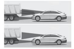
• When a vehicle ahead disappears at an intersection, your vehicle may accelerate.
