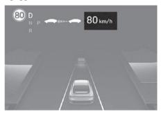
Manual Speed Limit Assist or Smart Cruise Control assists the vehicle to adjust its speed according to the speed limit. When the cruising speed is set as same as the speed limit, the vehicle automatically adjusts its speed if the speed limit changes. The function operates on the road which has a speed limit of 70 km/h (44 mph) or higher. When the function is active, the cruising speed on the instrument cluster appears in green.
