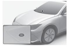
Never place anything near the ambient light/solar sensor to ensure better control of the heating and cooling system.
