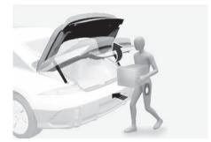
On a vehicle equipped with a smart key, the trunk can be opened with hands-free activation using the smart trunk system.
