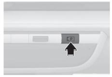
1 With the vehicle turned on, depress the brake pedal and shift the gear to P (Park) or N (Neutral).
