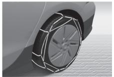
Since the sidewalls of radial tires are thinner than other types of tires, they may be damaged by mounting some types of tire chains on them. Therefore, the use of snow tires is recommended instead of tire chains. If tire chains must be used, use genuine HYUNDAI parts and install the tire chain after reviewing the instructions provided with the tire chains. Damage to your vehicle caused by improper tire chain use is not covered by your vehicle manufacturer's warranty.
