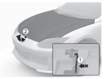
3. Go to the front of the vehicle, raise the hood slightly, push to the left the secondary hood release lever (1) inside of the hood center and lift the hood (2).
