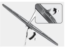
1 Lift up the wiper blade clip (1). Then lift up the wiper blade.
