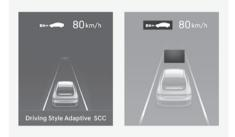
When Based on Driving Style is operating, "Driving Style Adaptive SCC" message will appear on the cluster for 2 seconds, and the distance level and target distance will be displayed based on the driving style.
