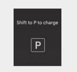
This message is displayed if you connect the charging cable without the gear in the P (Park) position.
