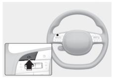
Press the Driving Assist (CC) button to turn Manual Speed Limit Assist off. The Speed Limit (GLIMIT) indicator will go off.
