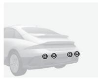
[A] Front ultrasonic sensors, [B] Rear ultrasonic sensors
