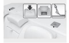
Top-tether anchorages for Child Restraint Systems are located on the rear of the seatbacks.
