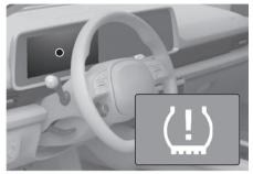
The TPMS Malfunction Indicator will illuminate after it blinks for about one minute when there is a problem with the Tire Pressure Monitoring System.
