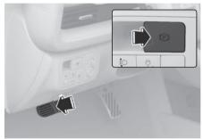
To release EPB (Electronic Parking Brake):
