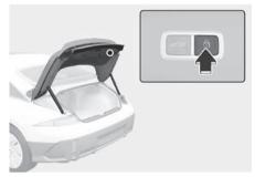
Press the power trunk lock button while carrying the smart key. The power trunk will close and lock with a warning sound. Additionally, all doors will lock. The trunk will close and lock, and all doors will lock only when the vehicle is off or all doors are closed.
