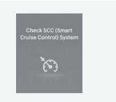
When Smart Cruise Control is not working properly, the 'Check Smart Cruise Control System' (or 'Check SCC (Smart Cruise Control) system') warning message will appear, and the ( $\triangle$ ) warning light will illuminate on the instrument cluster. We recommend that you have the vehicleinspected by an authorized HYUNDAldealer.
