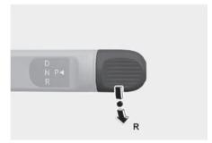
To shift the gear to R (Rear), rotate the rotary gear shift dial to R (Reverse) while depressing the brake pedal.
