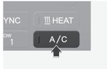
Touch the CLIMATE icon in the climate control panel. The climate information screen will appear on the infotainment screen. Touch the A/C icon in the infotainment screen to turn the air conditioning on (indicator light ON) and off.
