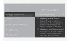
With the vehicle on, select or deselect "Setup (Settings) > Vehicle > Driver assistance > Driving convenience" from the Settings menu to set whether to use each function.
