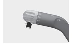
To turn on the high beam headlamp, push the lever away from you. The lever will return to its original position.
