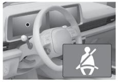
As a reminder to the driver, the driver's seat belt warning lights will illuminate for about 6 seconds each time the START/STOP button is in the ON position regardless of belt fastening. If the seatbelt is not fastened, the warning chime will sound for about 6 seconds.
