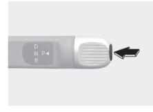
To shift the gear to P (Park), press the P button while depressing the brake pedal.
