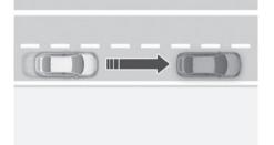
Highway Lane Change Assist (if equipped) Highway Lane Change Assist function helps change lanes to the direction the driver slightly moves the turn signal switch if the function judges that lane change is possible.
