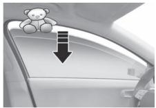
If a window senses any obstacle while it is closing automatically, it will stop and lower about 30 cm (12 in.) to allow the object to be cleared.
