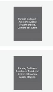
The "Parking Collision-Avoidance Assist system limited. Camera obscured" or "Parking Collision-Avoidance Assist syst. limited. Ultrasonic sensor blocked" warning message will appear on the cluster if the following situations occur:
