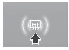
The defroster heats the window to remove frost, fog and thin ice from the interior and exterior of the rear window, while the vehicle is running.
