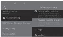
With the vehicle on, select "Setup (Settings) > Vehicle > Driver assistance > Warning volume" from the Settings menu to change the Warning Volume to "High", "Medium" or "Low" for Intelligent Speed Limit Assist.
