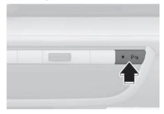
Turning Parking Collision Avoidance Assist On/Off
