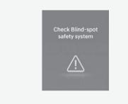
When Blind-Spot Collision Warning is not working properly, the "Check Blind-spot safety system" warning message will appear on the instrument cluster for several seconds, and the master ( $\triangle$ ) warning light will illuminate on the instrument cluster. If this occurs, we recommend that you have the vehicle inspected by an authorized HYUNDAI dealer.
