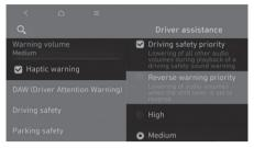
With the vehicle on, select **"Setup** (Settings) > Vehicle> Driver assistance > Warning Volume" from the Settings menu to change the Warning Volume for Lane Keeping Assist.
