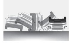
Front airbags may not inflate in rollover accidents because front airbag deployment would not provide additional occupant protection.
