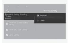
With the vehicle on, select 'Setup (Settings) > Vehicle > Driver assistance > Driving safety > Forward safety warning timing' from the Settings menu to change the initial warning activation time for Forward Collision Avoidance Assist. The warning time can be set to either 'Standard (Normal)' or 'Late (Later)'.
