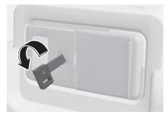
3. Open the power outlet cover by sliding it to the left, and connect the power plug of the electric device to the power socket.
