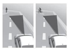
Forward Collision-Avoidance Assist may not detect other vehicles, powered two-wheelers pedestrians or cyclists in front of you when driving on curved roads adversely affecting the performance of the sensors. This may result in no warning, braking assist or steering assist (if equipped) when necessary.
