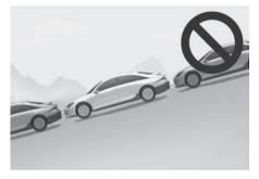
Park or exit manually when the vehicle is on inclines.
