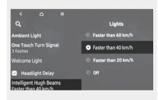
With the Start/Stop button in the ON position, select 'Setup > Vehicle Settings > Lights > Intelligent High Beams' from the Settings menu to turn on Intelligent Front-Lighting System and deselect to turn off the system.
