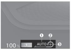
The instrument cluster displays 'AUTO' (1) when the smart recuperation system is ON. Depending on the conditions, the system adjusts the regenerative braking level (2). The sky blue indicator light (3) illuminates when the vehicle recognizes a vehicle.
