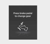
This message is displayed when the brake pedal is not depressed while shifting the gear.
