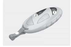
You can still control the window movement with the vehicle turned off by pressing the Door Lock button (1) or the Door Unlock button (2).
