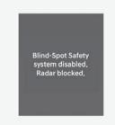
When the rear bumper around the rear corner radar or sensor is covered with foreign material, such as snow or rain, or installing a trailer or carrier, it can reduce the detecting performance and temporarily limit or disable Safe Exit Assist.
