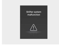
This message is displayed when the shift gear does not properly operate in the P (Park) position.
