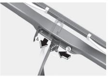
2. Press the clip (3). Then push the blade forward through the wiper arm to disassemble it (4).
