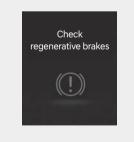
These warning messages are displayed when the regenerative brake system does not work properly. In this case, we recommend that you have the vehicle inspected by an authorized HYUNDAI dealer.
