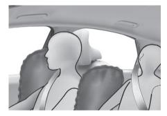
Your vehicle is equipped with a side airbag in each front seat. The purpose of the airbag is to provide the vehicle's additional protection than that offered by the seat belt alone.
