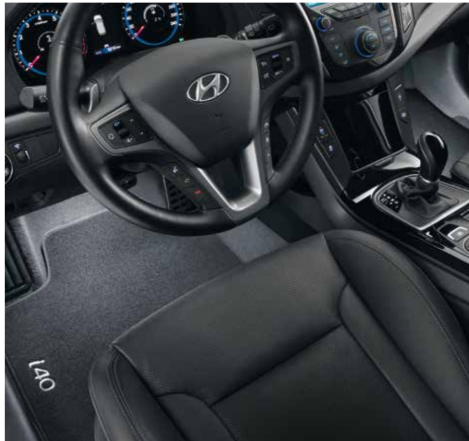
White LED lighting foot area. Concealed floor illumination for the front foot space. It provides welcome illumination that automatically switches on and off with the opening and closing of the front doors. Upon starting the engine the illumination dims out. Also available for the second row of the vehicle. Second row only in combination with first row LED lighting. 99650ADE00W (first row/MY11, MY15/Sedan, Wagon), 99650ADE10W (second row/MY11, MY15/Sedan, Wagon)
