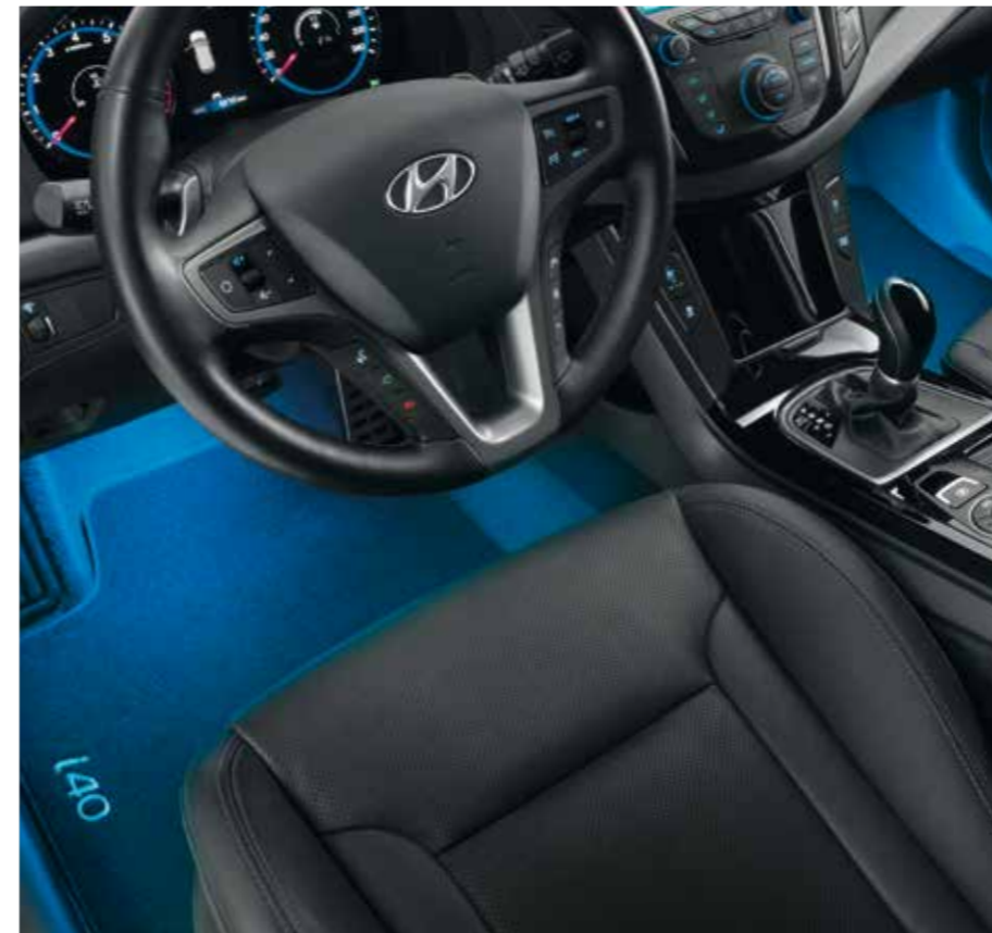
Blue LED lighting foot area. Concealed floor illumination for the front foot space. It provides welcome illumination that automatically switches on and off with the opening and closing of the front doors. Upon starting the engine the illumination dims out. Also available for the second row of the vehicle. Second row only in combination with first row LED lighting. 99650ADE00 (first row/MY11, MY15/Sedan, Wagon), 99650ADE10 (second row/MY11, MY15/Sedan, Wagon)
