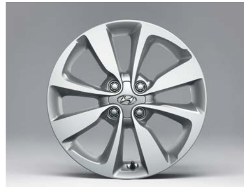
Alloy wheel 16". Eight-spoke alloy wheel, bicolour, 6,0Jx16, suitable for 195/55 R16 tyres. Cap and nuts are not included. LP52910C8100 (5dr)
