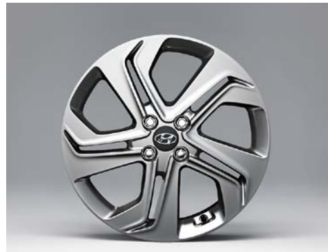
Alloy wheel 17". Five-double-spoke alloy wheel, silver, 6,5Jx17, suitable for 205/45 R17 tyres. Cap and nuts are not included. LP52910C8200 (Coupé, Active)
