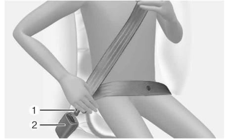
Pull the belt out of the retractor and insert the metal tab (1) into the buckle (2). There is an audible “click” sound when the tab locks into the buckle. Make sure the seat belt is not twisted.
