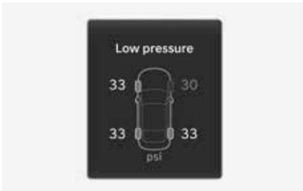
The tire pressure of each tire appears. For more information, refer to "Tire pressure monitoring system (TPMS) (Except Europe) " section in chapter 8.
