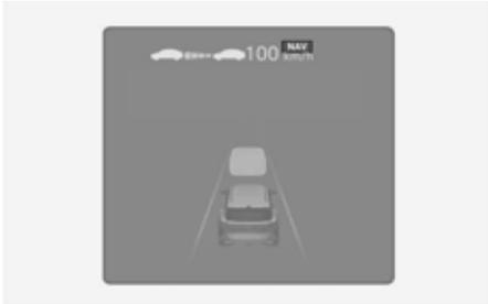
While the speed is being controlled, the green **NAV** indicator light blinks.
