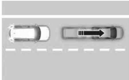
If the vehicle in front abruptly departs, Leading Vehicle Departure Alert may not operate properly.
