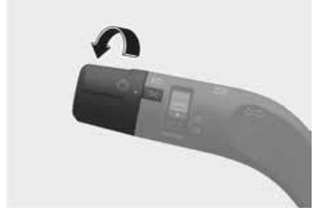
The position light, license plate light and instrument panel lamp are turned ON.
