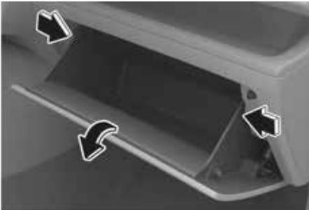
2. Open the glove box and remove the support rod (1).
