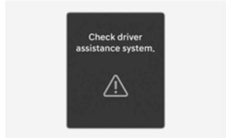
When Safe Exit Warning is not working properly, the "**Check Driver Assistance system**" warning message will appear on the cluster for several seconds, and the master warning light (
