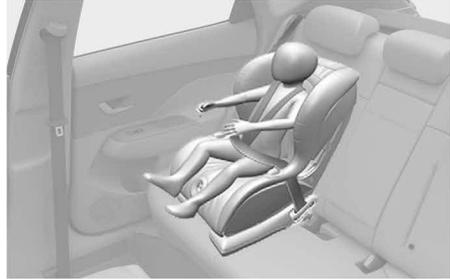
A forward-facing Child Restraint System provides restraint for the child's body with a harness. Keep children in a forward-facing Child Restraint System with a harness until they reach the top height or weight limit allowed by your Child Restraint System's manufacturer.
