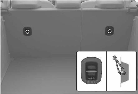
First secure the child restraint with the ISOFIX anchorages or the seat belt. If the child restraint manufacturer recommends that the top tether strap be attached, attach and tighten the top tether strap to the top tether strap anchorage.
