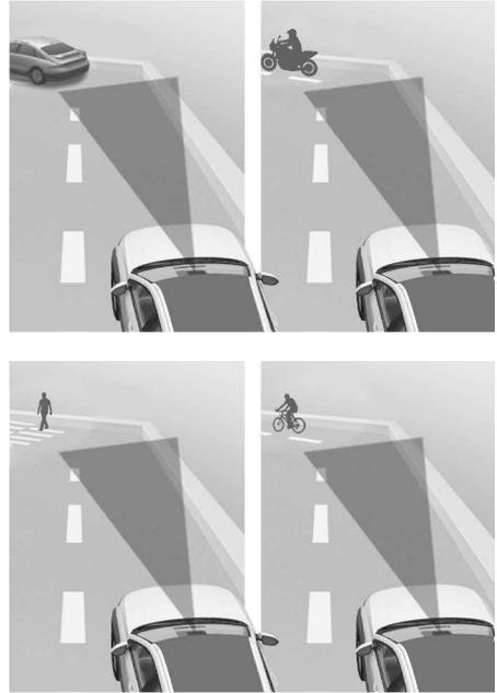
Forward Collision-Avoidance Assist may not detect a vehicle, a powered two wheeler, a pedestrian or a cyclists in front of you when driving on curved roads adversely affecting the performance of the sensors. This may result in no warning, braking assist when necessary.
