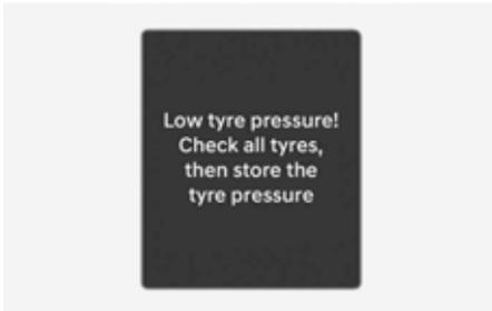
When the Low Tire Pressure warning light (⚠️) illuminates and a warning message appears on the cluster for 10 seconds, one or more of your tires is significantly under-inflated.
