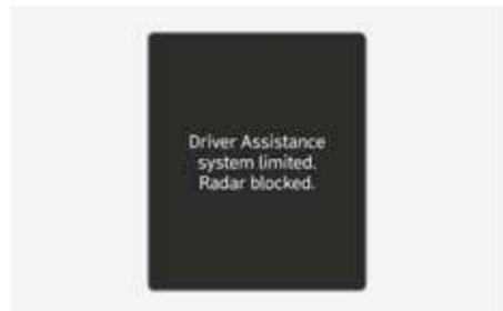
When the front windshield where the front view camera is located, front radar cover, or sensor is covered with foreign material, such as snow or rain, it can reduce the detecting performance and temporarily limit or disable Forward Collision-Avoidance Assist.
