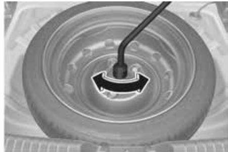
If it is hard to loosen the tire hold down wing bolt by hand, you can loosen it easily using the wheel lug wrench.
