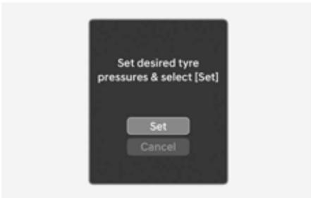
5. Check whether the "**Standard tyre pressures saved**" message appears on the cluster and the
