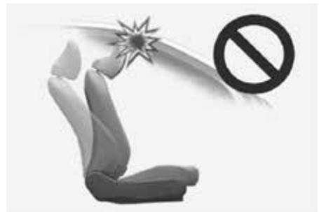
If you recline the seatback towards the front with the headrest and seat cushion raised, the headrest may come in contact with the sunvisor or other parts of the vehicle.
