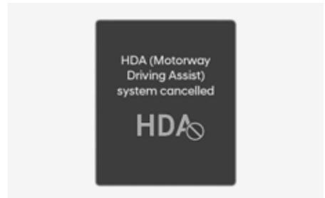
If the driver still does not have their hands on the steering wheel after the hands-off warning, **"HDA(Motorway Driving Assist) system cancelled"** warning message will appear and Highway Driving Assist and Lane Change Assist will be automatically cancelled.
