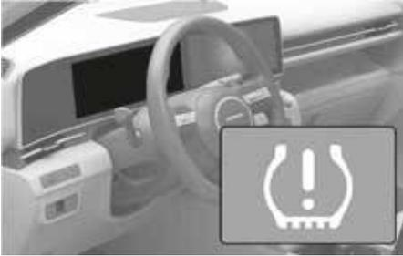
The TPMS Malfunction Indicator (⚠️) illuminates after it blinks for approximately one minute when there is a problem with the Tire Pressure Monitoring System.
