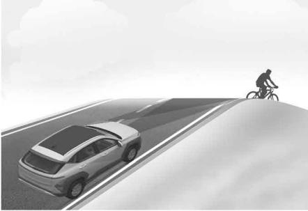
Forward Collision-Avoidance Assist may not detect a vehicle, a powered two wheeler, and a pedestrian or a cyclist in front of you while driving uphill or downhill, adversely affecting the performance of the sensors.
