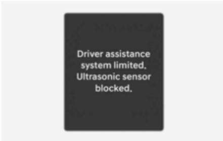
If this occurs the **"Driver Assistance system limited. Ultrasonic sensor blocked"** warning message appears on the instrument cluster. Parking Distance Warning will operate properly when snow, rain or foreign material is removed. If Parking Distance Warning does not operate properly after obstruction (snow, rain, or foreign material) is removed (including trailer, carrier, etc., from the rear bumper), we recommend that you contact an authorized HYUNDAI dealer.
