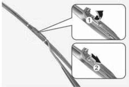
4. Install a new wiper blade assembly in the reverse order of removal.
