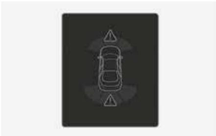
When the Parking Distance Warning is operating, if the function is not working normally or the ultrasonic sensor is blocked, the master warning light (▲) appears in the direction of the corresponding sensor. You can check the warning in the Utility view on the cluster.
