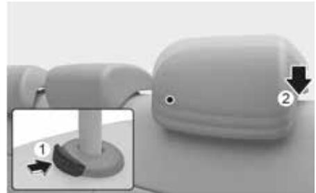
1. Put the headrest poles into the holes (3) while pressing the release button (1).
