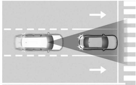
Forward Collision-Avoidance Assist detects a vehicle, a powered-two wheeler, a pedestrian, or a cyclist ahead on the road and may warn you of a possible collision with a warning message on the instrument cluster and a warning sound. Also, Forward Collision-Avoidance Assist may assist with braking your vehicle to help reduce collision speed or avoid a collision.
