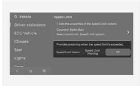
With the vehicle on, select or deselect **Settings > Vehicle > Driver Assistance > Speed Limit** from the Settings menu to set whether to use each function.
