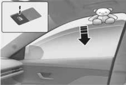
If a window senses any obstacle while it is closing automatically, it will stop and lower about 30 cm (12 in.) to allow the object to be cleared.
