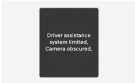
When the front windshield where the front view camera is located or the sensor is covered with foreign material, such as snow or rain, it can reduce the detecting performance and temporarily limit or disable Forward Collision-Avoidance Assist.
