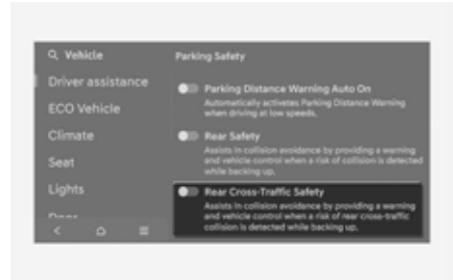
With the vehicle on, select **Settings** > **Vehicle** > **Parking Safety** > **Rear Cross-Traffic Safety** from the settings menu in the infotainment system to turn on Rear Cross-Traffic Collision-Avoidance Assist and deselect to turn off the function.
