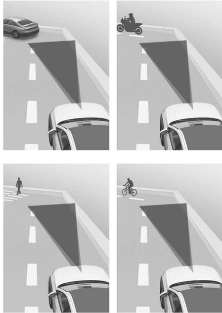
Forward Collision-Avoidance Assist may not detect a vehicle, a powered two wheeler, and a pedestrian or a cyclist in front of you when driving on curved roads adversely affecting the performance of the sensors. This may result in no warning, braking assist when necessary.
