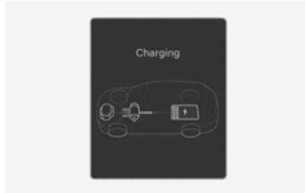
The engine charges up the high voltage battery. The motor power is used to drive the vehicle.
