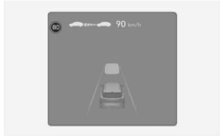
When driving at a speed higher than the displayed speed limit, the red speed limit indicator will blink and warning sounds.
