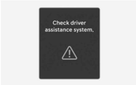
When Lane Keeping Assist is not working properly, the "**Check Driver Assistance system**" warning message and yellow Lane Keeping Assist (LKA) warning light appears on the cluster. If this occurs, we recommend that your vehicle be inspected by an authorized HYUNDAI dealer.
