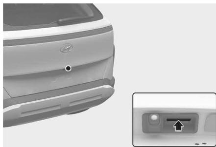
2. Start the vehicle within 30 seconds after pressing the **12V BATT RESET** button.
