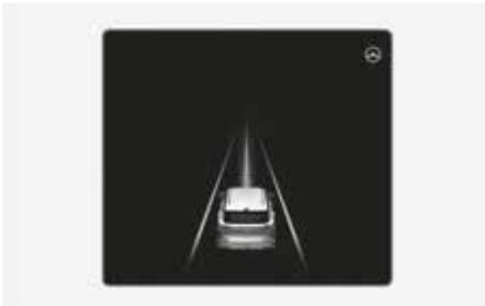
If the vehicle ahead and/or both lane markings are detected and your vehicle speed is below 200 km/h (120 mph), the green (S) indicator light appears on the cluster, and Lane Following Assist helps center the vehicle in the lane by assisting the steering wheel.
