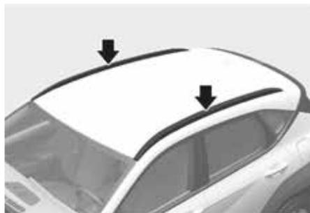
Your vehicle may come equipped with roof side rails. If your vehicle is equipped with roof rack rails, you can add roof rack crossbars as an accessory (not shown).
