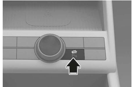
Press the Parking Safety (P<sub>W</sub>) button to turn on Forward/Reverse Parking Distance Warning. Press the button again to turn off the function.
