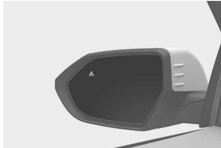
Your vehicle is equipped with both left-hand and right-hand outside rearview mirrors. The mirrors can be adjusted with the mirror adjustment control switch. Adjust the side view mirrors to your desired position before driving. The outside rearview mirrors can be folded to help prevent damage when going through an automatic car wash or when passing through a narrow street.
