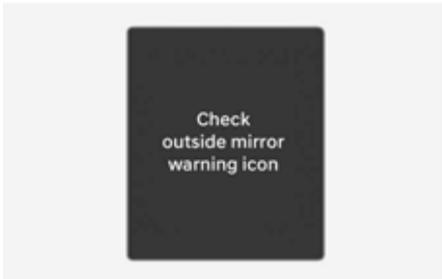
When the outside rearview mirror warning light is not working properly, the **"Check side view mirror warning light"** (or **"Check outside mirror warning icon"**) warning message will appear on the instrument cluster for several seconds, and the master (▲) warning light will illuminate on the cluster. If this occur, we recommend that your vehicle be inspected by an authorized HYUNDAI dealer.
