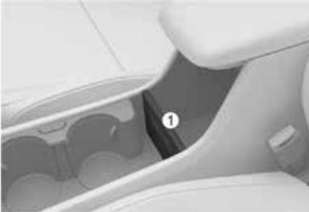
The removable partition (1) can be removed to expand the storage compartment.
