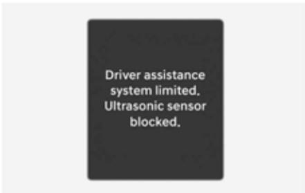
The "**Driver Assistance system limited. Camera blocked**" or "**Driver Assistance system limited. Ultrasonic sensor blocked**" warning message will appear on the cluster if the following situations occur:
