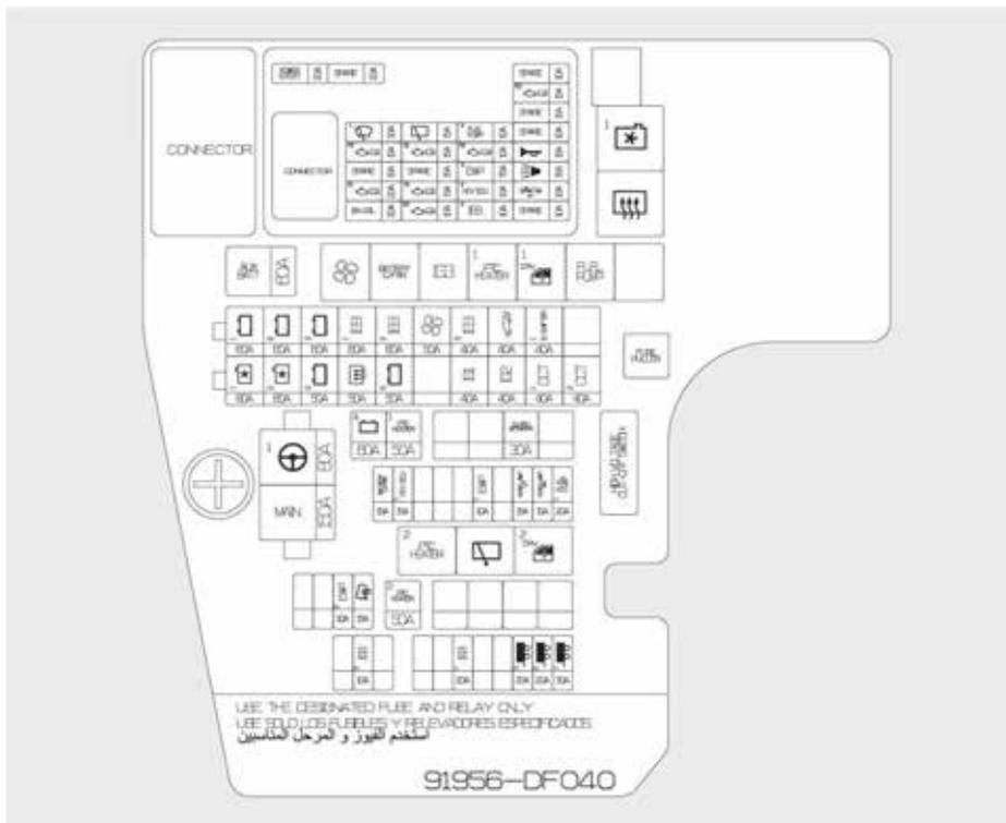
Engine compartment fuse panel (Engine compartment junction block)
