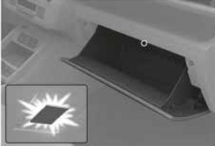
The glove box lamp turns on when the glove box is opened.
