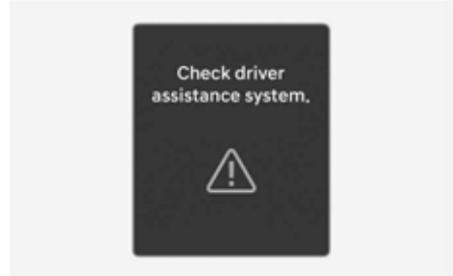
When Reverse Parking Collision-Avoidance Assist or other related functions are not working properly, the "**Check Driver Assistance system**" warning message will appear on the instrument cluster, and Reverse Parking Collision-Avoidance Assist will turn off automatically. We recommend that your vehicle be inspected by an authorized HYUNDAI dealer.
