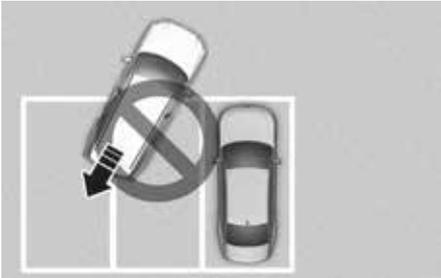
If Remote Smart Parking Assist is used, when parking in a parking space with a vehicle only on one side, your vehicle may cross the parking line to avoid the parked vehicle.
