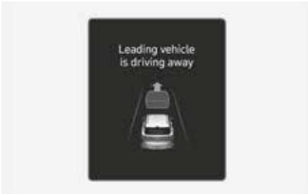
When a detected vehicle in front departs from a stop, Leading Vehicle Departure Alert will inform the driver by displaying the "**Leading vehicle is driving away**" message on the instrument cluster and an audible warning will sound.
