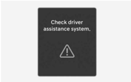
When Smart Cruise Control is not working properly, the "**Check Driver Assistance system**" warning message and the master (⚠) warning light will appear on the instrument cluster. We recommend that your vehicle be inspected by an authorized HYUNDAI dealer.
