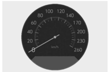
The speedometer indicates the speed of the vehicle and is calibrated in kilometers per hour (km/h) and/or miles per hour (MPH).
