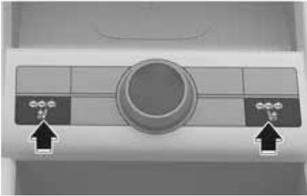
While the engine running, press the switches to cool the driver's seat or front passenger's seat.
