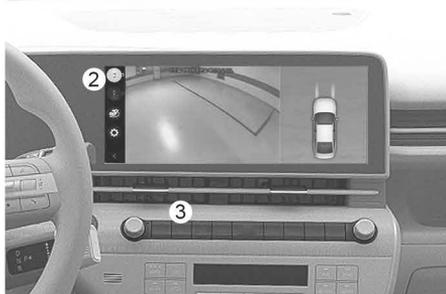
The front view appears on the screen when the gear is in N (Neutral) or D (Drive) to assist in parking.
