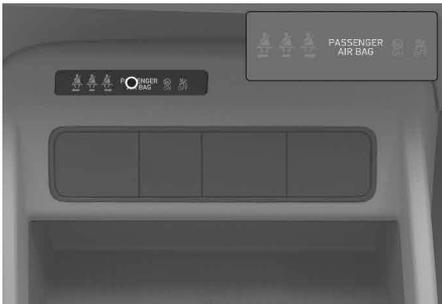
Insert the key or a similar rigid device into the passenger's front airbag ON/ OFF switch and turn it to the OFF position [B]. The passenger airbag OFF indicator (⚡) illuminates and stays on until the passenger's front airbag is reactivated.
