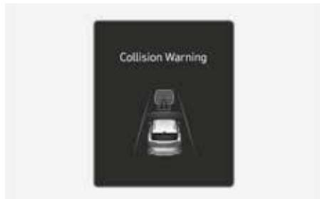
While Smart Cruise Control is operating, when the collision risk with the vehicle ahead is high, the 'Collision Warning' warning message will appear on the instrument cluster, and an audible warning will sound to warn the driver. Always have your eyes on the road while driving, and if necessary, depress the brake pedal to reduce your driving speed in order to maintain a safe distance.
