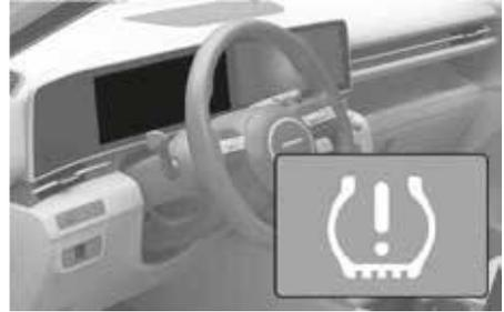
The TPMS malfunction indicator (ⓘ) illuminates after blinking for about 70 seconds when there is a problem with the Tire Pressure Monitoring System.
