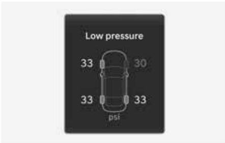
When the tire pressure monitoring system warning indicator (⚠️) is illuminated and a warning message displayed on the cluster display, one or more of your tires is significantly under-inflated. The Low Tire Pressure Position Telltale will indicate which tire is significantly under inflated by illuminating the corresponding position light.
