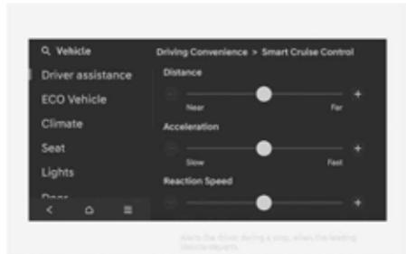
With the vehicle on, select **Settings > Vehicle > Driver Assistance > Driving Convenience > Smart Cruise Control** from the settings menu in the infotainment system to change Distance, Acceleration, Reaction Speed manually.
