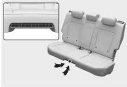
The hybrid battery cooling duct is located below the center of the rear seat. The cooling duct cools down the hybrid battery. When the hybrid battery cooling duct is blocked, the hybrid battery may be overheated.
