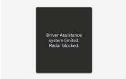
When the rear bumper around the rear corner radar or sensor is covered with foreign material, such as snow or rain, or installing a trailer or carrier, it can reduce the detecting performance and temporarily limit or disable Safe Exit Warning.
