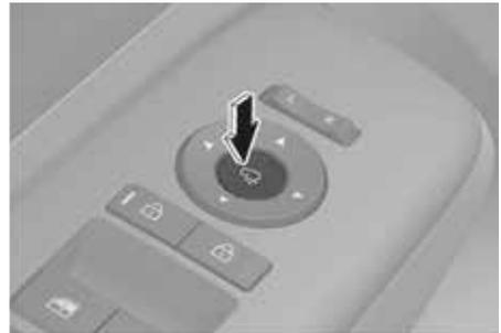
The outside rearview mirrors can be folded or unfolded by pressing the button.
