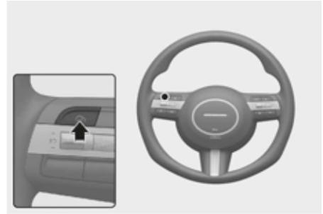
To turn Smart Cruise Control off, press the Driving Assist (
