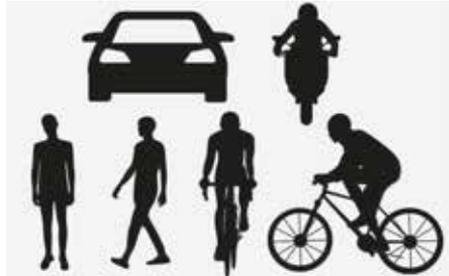
The illustration above shows the image the front view camera is capable of detecting as a vehicle, powered two wheeler, pedestrian, and cyclist.
