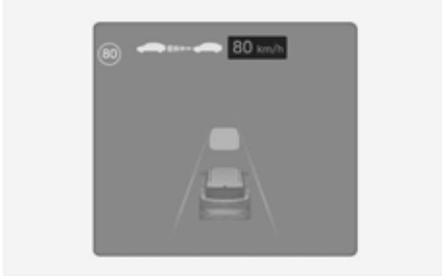
Manual Speed Limit Assist or Smart Cruise Control assists the vehicle to adjust its speed according to the speed limit. When the cruising speed is set as same as the speed limit, the vehicle automatically adjusts its speed if the speed limit changes. The function operates on the road which has a speed limit of 70 km/h (44 mph) or higher. When the function is active, the cruising speed on the instrument cluster appears in green.
