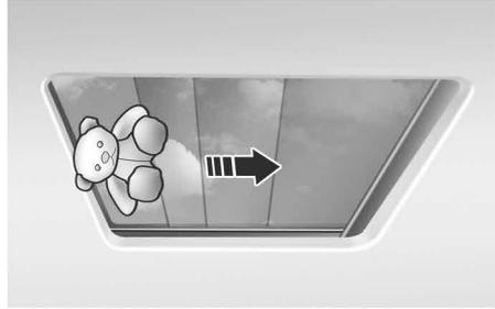
If the power sunshade or sunroof glass senses any obstacle while it is closing automatically, it reverses direction then stops.
