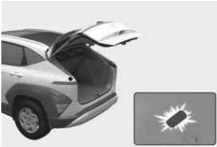
The cargo area lamp turns on when the tailgate is opened and off when the tailgate is closed.
