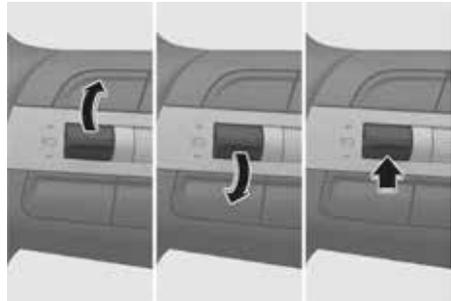
To resume Manual Speed Limit Assist after the function was paused, operate the +, -,
