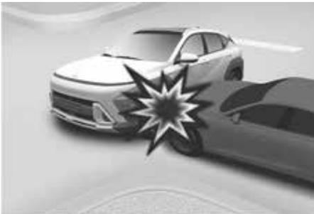
Front airbags may not inflate in side impact collisions, because occupants move in the direction of the collision.
