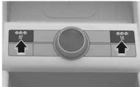
While the engine is running, press the switch to warm the driver's seat or front passenger's seat.
