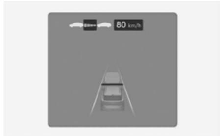
If you want to speed up temporarily without altering the set speed while Smart Cruise Control is operating, depress the accelerator pedal. While the accelerator pedal is depressed, the set speed, distance level and target distance will blink on the cluster.
