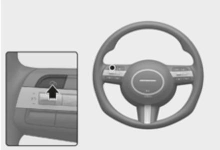
Press the Driving Assist (
