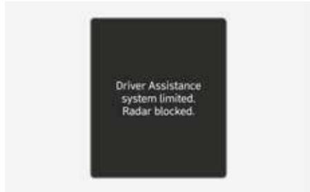
When the front radar cover or sensor is covered with snow, rain, or foreign material, it can reduce the detecting performance and temporarily limit or disable Smart Cruise Control.
