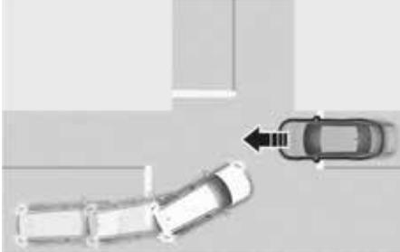
Junction Turning function can help avoid a collision with an oncoming vehicle in an adjacent lane when turning left (left-hand drive) or right (right-hand drive) at a crossroad with the turn signal on by applying emergency braking.
