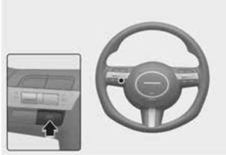
With the vehicle on, shortly press the Lane Driving Assist button located on the steering wheel to turn on Lane Following Assist. The grey or green (S) indicator light will appear on the cluster.
