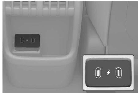
The USB charger is designed to recharge batteries of small size electronic devices using a USB cable.
