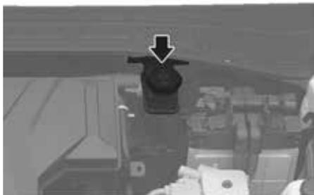
Check the fluid level in the reservoir periodically. The fluid level must be between the MAX and the MIN marks on the side of the reservoir.
