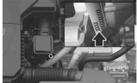
The engine number is stamped on the engine block as shown in the drawing.
