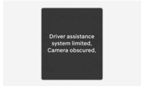
When the front windshield where the front view camera is located, or sensor is covered with foreign material, such as snow or rain, it can reduce the detecting performance and temporarily limit or disable Lane Keeping Assist.
