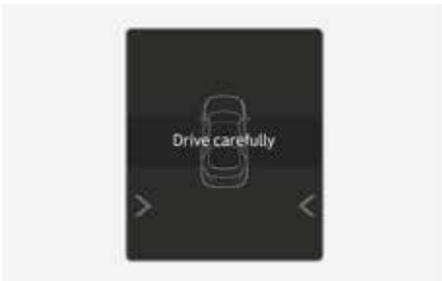
When the vehicle is stopped due to emergency braking, the 'Drive carefully' warning message will appear on the cluster.
