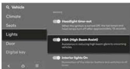
With the Engine Start/Stop button in the ON position, select **Vehicle>Lights > HBA (High Beam Assist)** from the Settings menu to turn on High Beam Assist and deselect to turn off the function.
