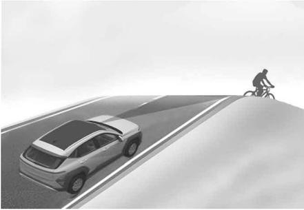
Forward Collision-Avoidance Assist may not detect a vehicle, a powered two wheeler, a pedestrian or a cyclists in front of you while driving uphill or downhill, adversely affecting the performance of the sensors.
