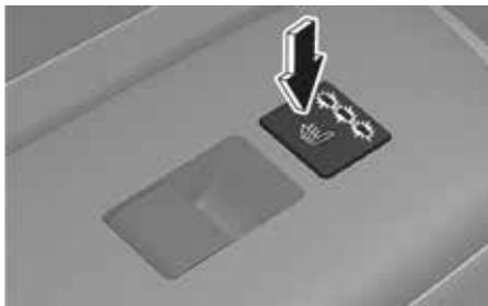
While the engine is running, press the seat warmer switch to warm the rear seat.
