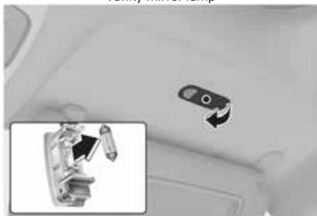
1. Using a flat-head screwdriver, gently pry the lens from the interior light housing.
