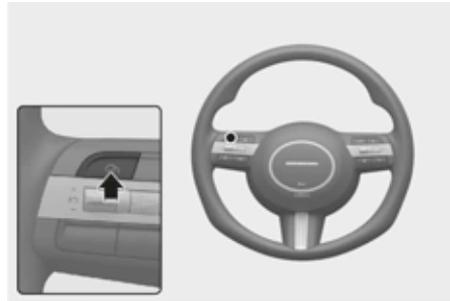
2. Press the Driving Assist button at the desired speed. The set speed and Cruise (CRUISE) indicator will illuminate on the cluster.
