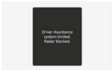
When the rear bumper around the rear corner radar or sensor is covered with foreign material, such as snow or rain, or installing a trailer or carrier, it can reduce the detecting performance and temporarily limit or disable Blind-Spot Collision-Avoidance Assist.
