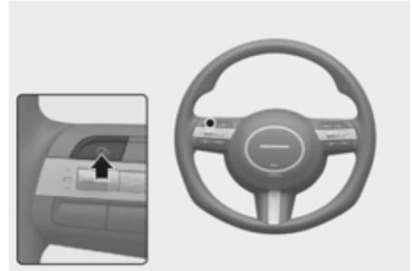
2. Push the + switch up or - switch down, and release it at the desired speed.
