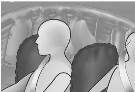
Side airbags are located in each front seat. Additionally, a front center side airbag is located in the inboard side of the driver seatback.
