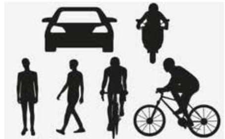
The illustration above shows the image the front view camera and front radar are capable of detecting as a vehicle, powered two wheeler, and pedestrian and cyclist.
