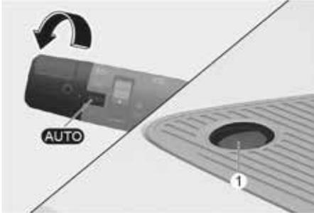
The position light and headlight may be turned ON or OFF automatically depending on the amount of daylight as measured by the ambient light sensor (1) at the upper end of the windshield glass.
