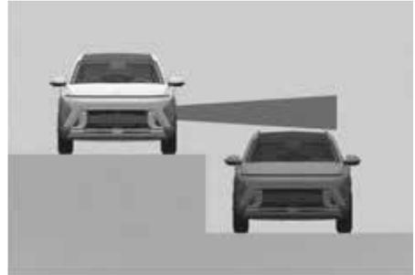
Blind-Spot Collision-Avoidance Assist may not operate properly when driving where the heights of the lanes are different. The function may not detect the vehicle on a road with different lane heights (underpass joining section, grade separated intersections, etc.). Always pay attention to road and driving conditions while driving.
