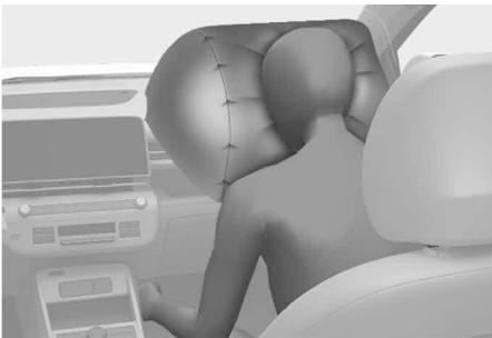
After complete inflation, the airbag immediately starts deflating, enabling the driver to maintain forward visibility and steer or operate other controls.
