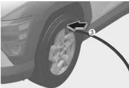
12. Plug the compressor power cord into the vehicle power outlet.
