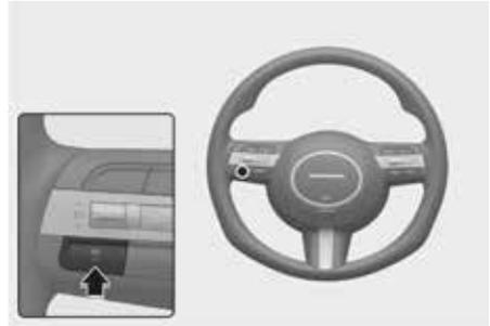
Press the button repeatedly to cycle through the headway settings from **Distance 4** → **Distance 3** → **Distance 2** → **Distance 1** → **Distance 4**.
