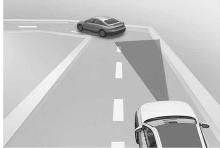
On curves, Smart Cruise Control may not detect a vehicle in the same lane, and may accelerate to the set speed. Also, vehicle speed may rapidly decrease when the vehicle ahead is detected suddenly.
