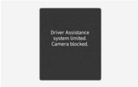
When the front windshield where the front view camera is located is covered with foreign material, such as snow or rain, it can reduce the detecting performance and temporarily limit or disable Intelligent Speed Limit Assist. If this occurs, the **"Driver Assistance system limited. Camera blocked"** warning message and the speed limit (⊖) warning light will appear on the instrument cluster.
