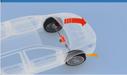
Mekaaninen kitkalukko Mechanical Limited Slip Differential (m-LSD)
